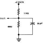
\*INCLUDING SCOPE AND JIG CAPACITANCE
