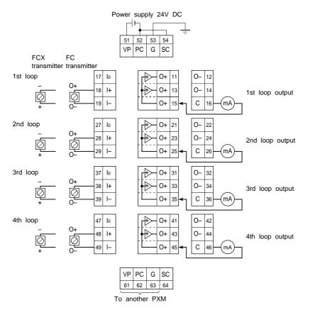
Note: 11 and 13 are connected to 15 output terminal with buffer amplifier,21 and 23 to 25,31 and 33 to 35, and 41and 43 to 45 respectively.
