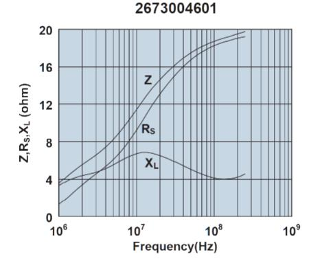
Impedance, reactance, and resistance vs. frequency.
