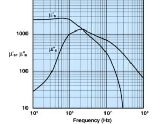
Measured on a 2673000301 bead using the HP 4284A and the HP 4291A.
