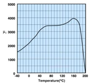
Measured on a 17/10/6mm toroid at 10kHz.
