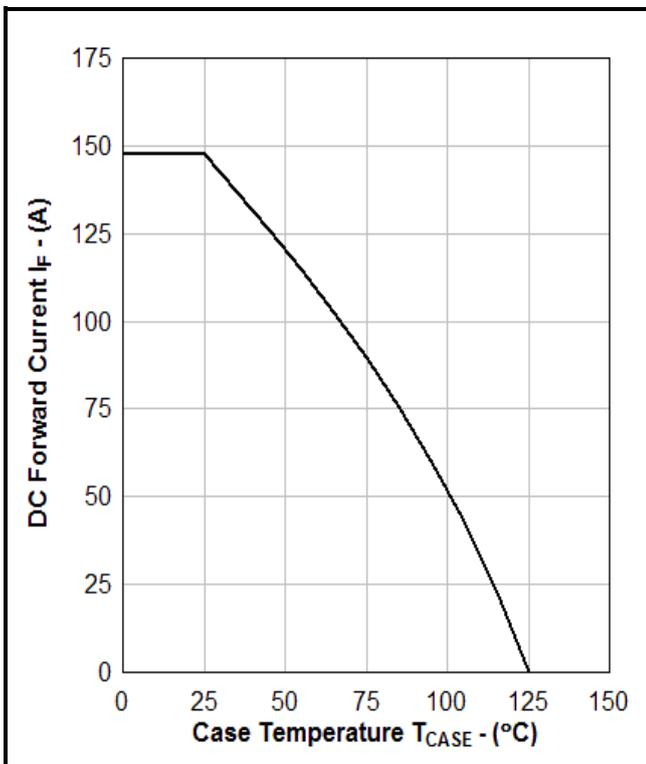
Fig. 5 DC current rating vs case temperature
