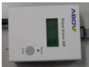
Figure 1-3 StandAlone ISP (VDD power is not supplied)
