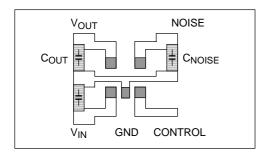
Circuit board material: glass epoxy, Circuit board dimension: 30 mm  $\times$  30 mm, Copper foil pad area: 50 mm<sup>2</sup> (t = 0.8 mm)
