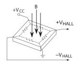
Figure 1. Hall element, basic circuit operation
