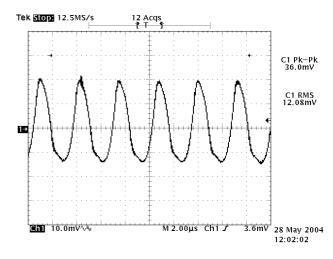
Figure 12: Output ripple & noise at 5.0Vin, 3.3V/10A out
