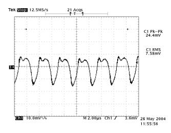
Figure 10: Output ripple & noise at 5.0Vin, 1.8V/10A out
