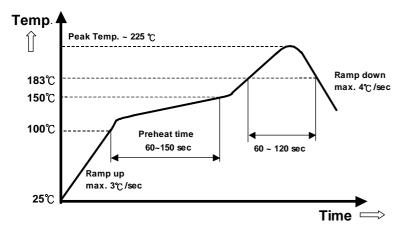
Note: All temperature refers to assembly application board, measured on the land of assembly application board.
