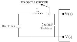
Note: Input reflected-ripple current is measured with a simulated source inductance. Current is measured at the input of the module.
