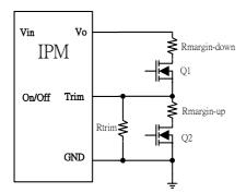
Figure 31: Circuit configuration for output voltage margining
