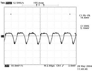
Figure 7: Output ripple & noise at 5.0Vin, 0.9V/10A out
