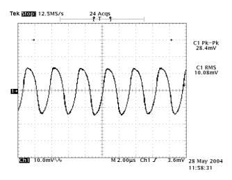
Figure 11: Output ripple & noise at 5.0Vin, 2.5V/10A out
