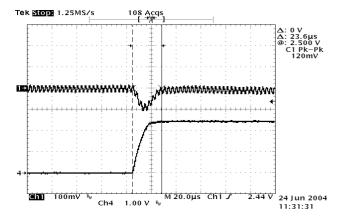
**Figure 21:** Typical transient response to step load change at 0.5A/μS from 0% to 50% of lo, max at 5.0Vin, 2.5V out (measurement with a 1uF ceramic and a 10μF tantalum
