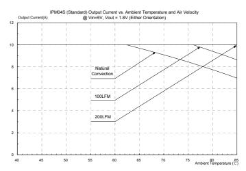
Figure 35: Output current vs. ambient temperature and air velocity @ Vin=5V, Vo=1.8V(either orientation)
