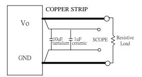
Note: Use a 10µF tantalum and 1µF capacitor. Scope measurement should be made using a BNC connector.
