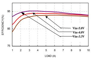
Figure 5: Converter efficiency vs. output current (2.5V 0utput voltage)
