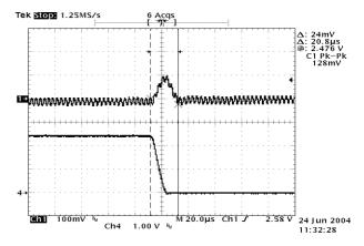
Figure 22: Typical transient response to step load change at 0.5A/μS from 50% to 0% of lo, max at 5.0Vin, 2.5V out (measurement with a 1uF ceramic and a 10μF tantalu)
