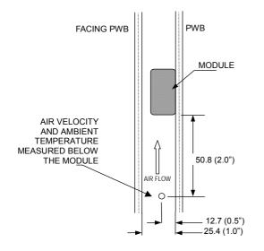
Figure 32: Wind tunnel test setup figure
