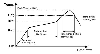
Note: All temperature refers to topside of the package, measured on the package body surface.
