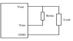
Figure 29: Trim down Circuit configuration for programming output voltage using an external resistor
