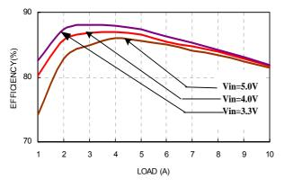
Figure 1: Converter efficiency vs. output current (0.90V output voltage)
