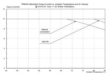
Figure 38: Output current vs. ambient temperature and air velocity @ Vin=3.3V, Vo=1.5V(Either Orientation) DS\_IPM04S0A010\_12182006
