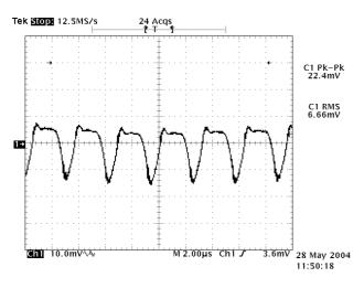
Figure 9: Output ripple & noise at 5.0Vin, 1.5V/10A out
