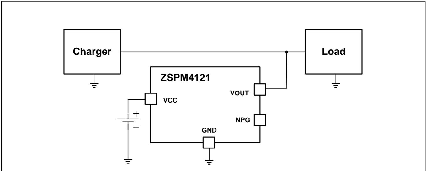
**Figure 4.2** Application Circuit for Disconnecting the Load
