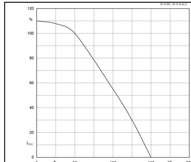
Fig. 2 : Rated forward current vs. ambient temperature
