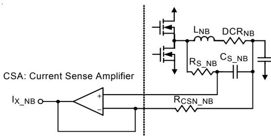
Figure 12. Current Sensing Circuit for NB Section
