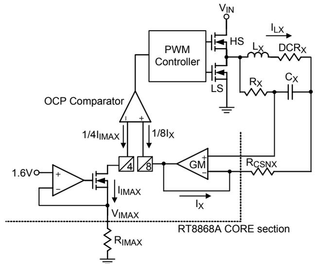
Figure 11. Over Current Protection for CORE Section
