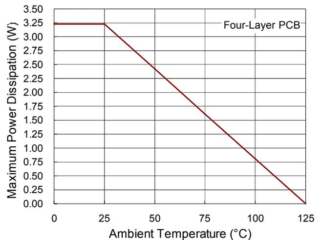
Figure 15. Derating Curve of Maximum Power Dissipation
