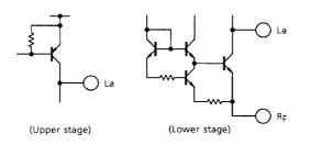
This circuit uses the power transistor's base current to regulate the circuit's output current. The upper-stage power transistor consists of a PNP discrete transistor (RN6006), which gives high torque efficiency.
