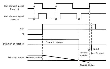
Note: Due to its inertial force, the motor does not stop immediately after the torque is reduced to 0.
