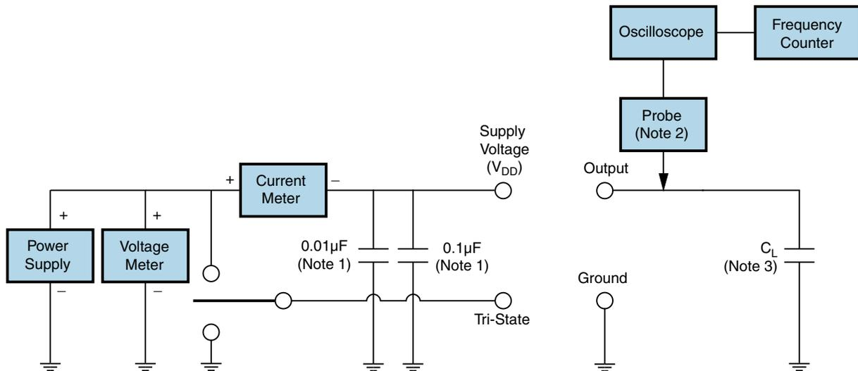
Note 1: An external 0.01 $\mu$ F ceramic bypass capacitor in parallel with a 0.1 $\mu$ F high frequency ceramic bypass capacitor close (less than 2mm) to the package ground and supply voltage pin is required.
