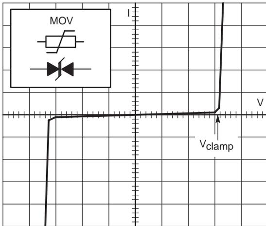
When a MOV reaches its Zener voltage, it starts to dissipate power, so this is why, if a high transient voltage occurs, the MOV may be damaged because of the high power dissipation that this transient may cause. At the same time, it is very common that the MOV becomes degraded each time it is activated.
