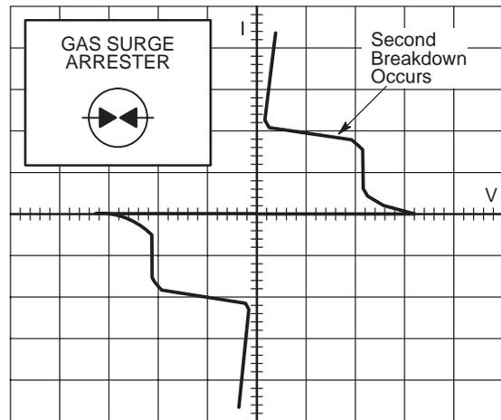
In this plot, it is possible to observe that the GDT’s response is relatively slow, and sometimes this factor could be very critical for telecom applications in which the fast response is needed. In addition, as a result of this slow response, some gas tubes’ electrodes burn out after a few hundred hits.
