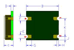
FR4 PCB Base: Solder masked All via holes tented on bottom Copper Clad ½ oz. Typical Gold plated 0.02 μinch (0.5 μm)
