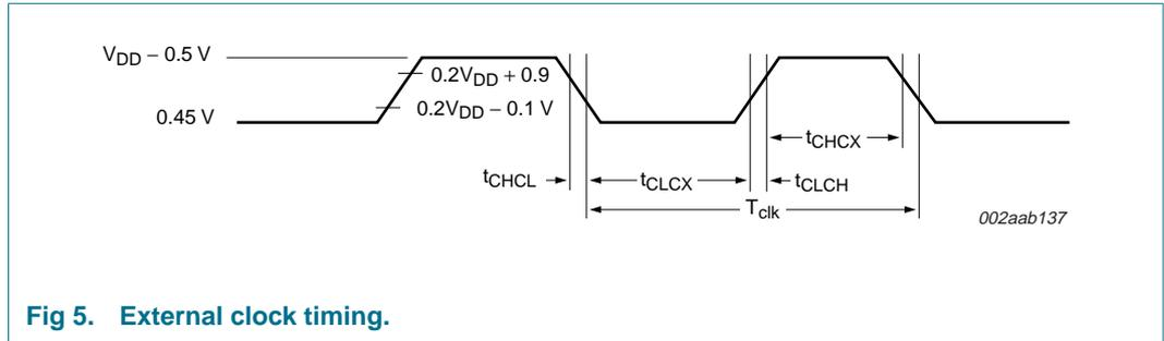
Fig 5. External clock timing.
