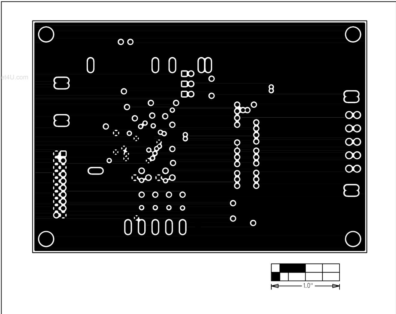
Figure 9. MAX1535 EV Kit PC Board Layout—Ground Plane
