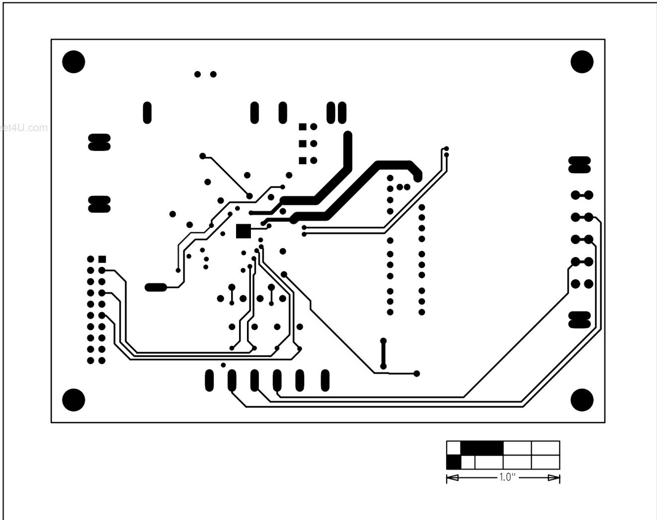
Figure 10. MAX1535 EV Kit PC Board Layout—Solder Side
