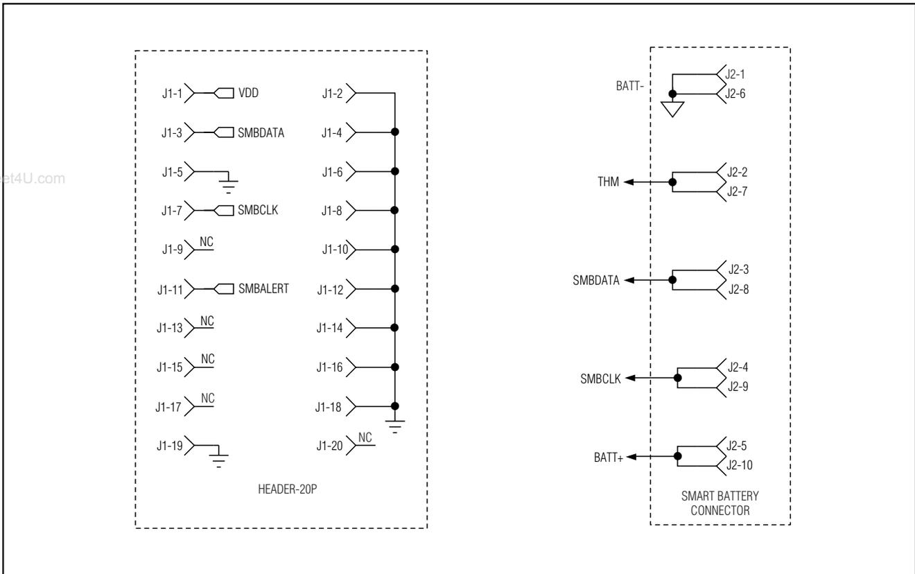
Figure 5. MAX1535 EV Kit Schematic—Smart Battery Connector
