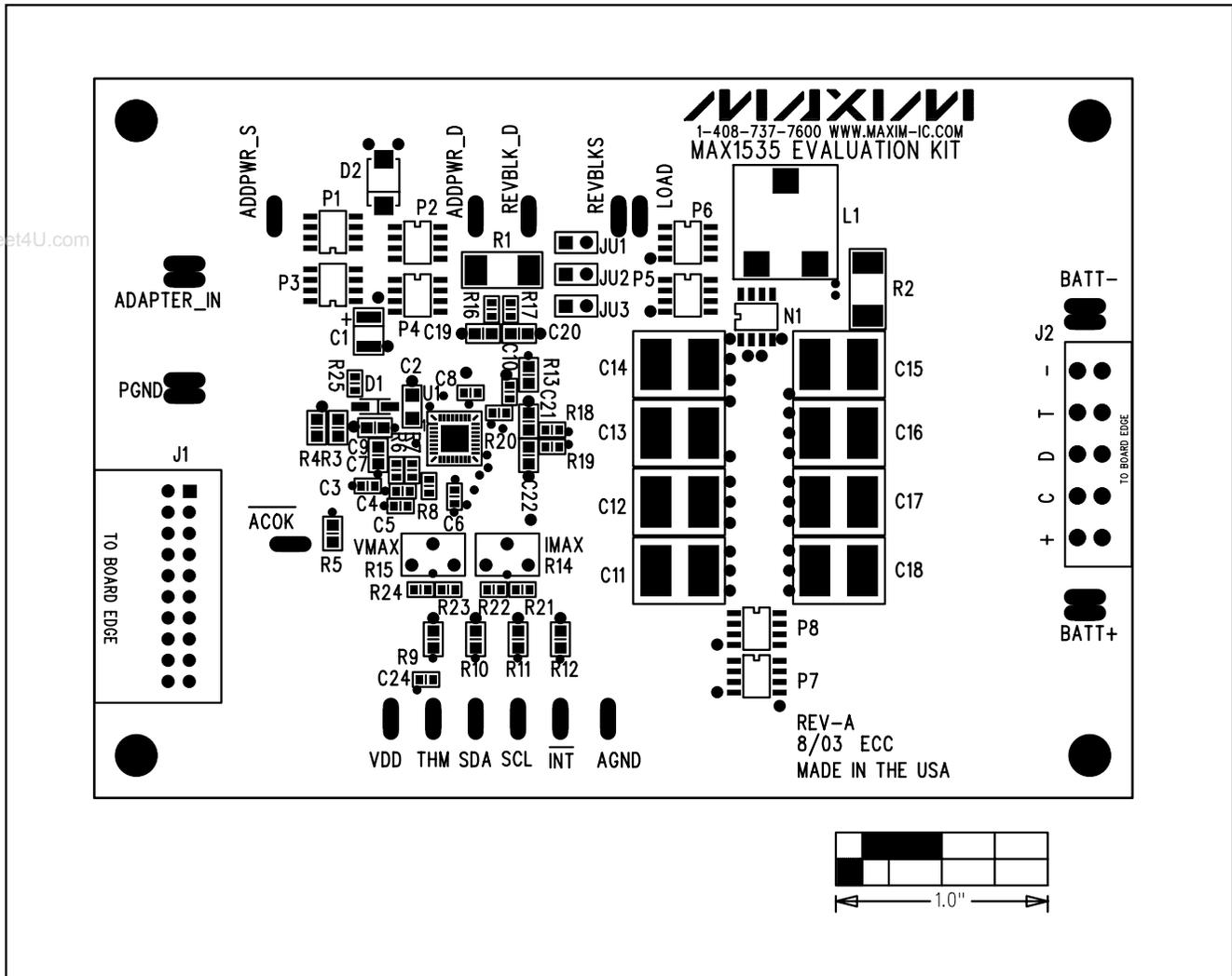
Figure 6. MAX1535 EV Kit Component Placement Guide—Component Side
