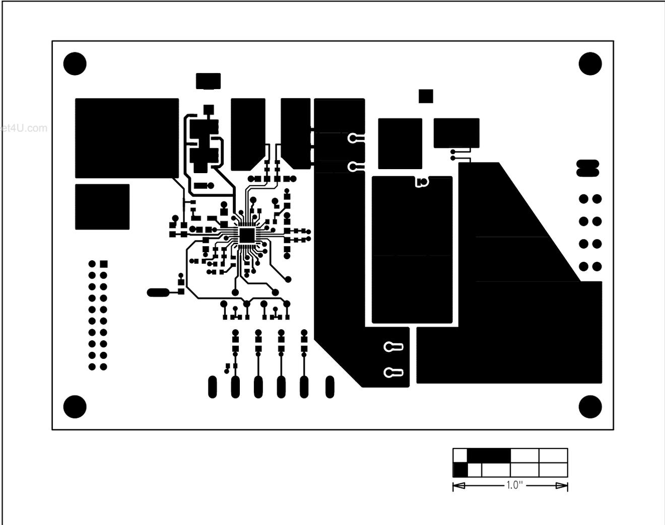
Figure 7. MAX1535 EV Kit PC Board Layout—Component Side
