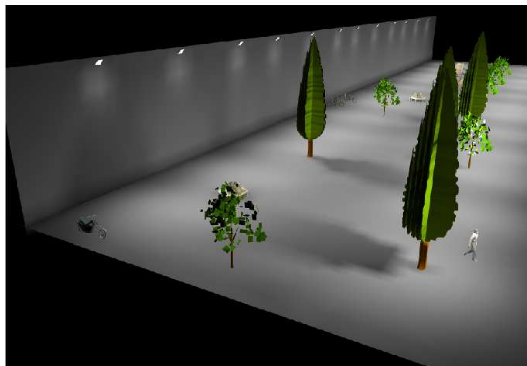
PHOTOMETRIC IMAGE OF WIDE OPTIC LED FLOODLIGHT
