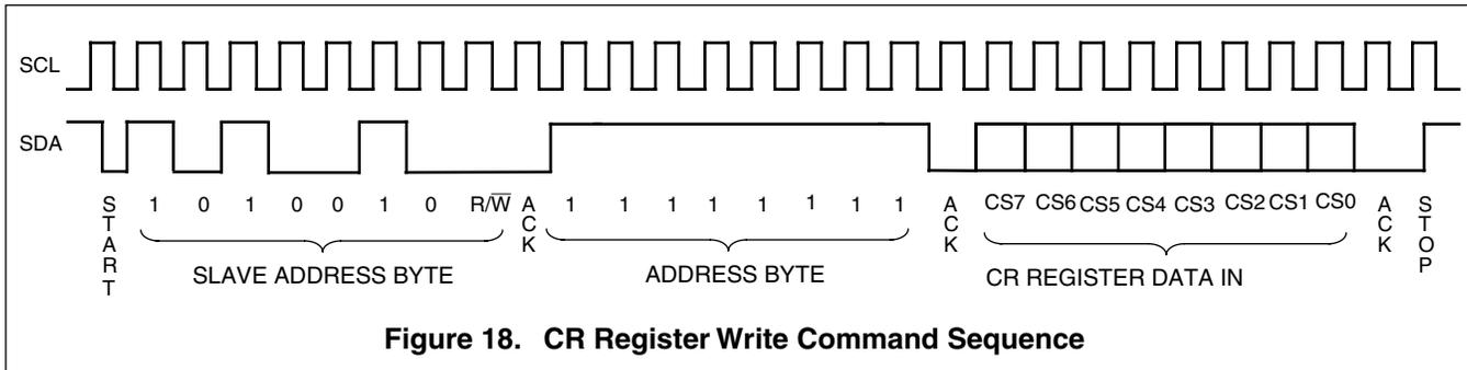
The region of EEPROM memory which is protected / locked is determined by the combination of the BL1 and BL0 bits written to the CR register. It is possible to lock the regions of EEPROM memory shown in the table below:
