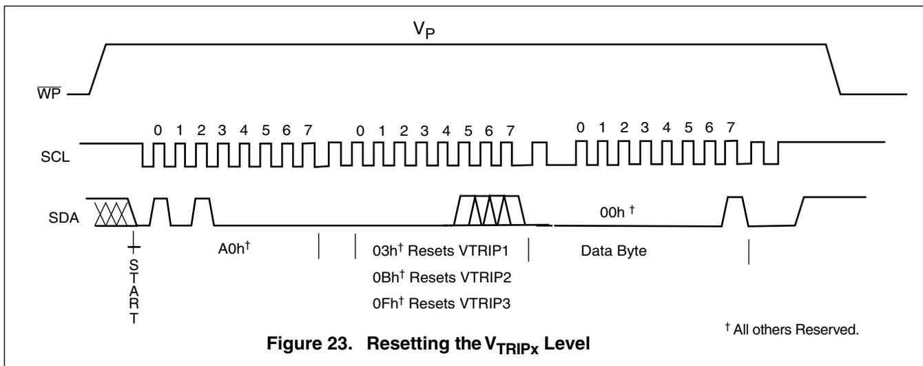
Figure 23. Resetting the  $V_{TRIPx}$  Level
