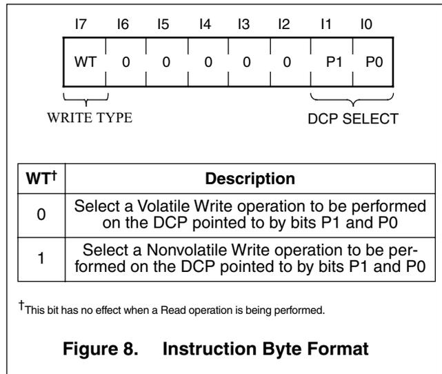
case, the two Least Significant Bit’s (I1 - I0) of the Instruction Byte are used to select the particular DCP (0 - 2). In the case of a Write to any of the DCPs (i.e. the LSB of the Slave Address is 0), the Most Significant Bit of the Instruction Byte (I7), determines the Write Type (WT) performed.
