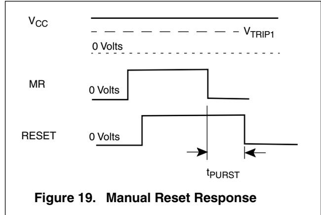
RESET remains HIGH for time  $t_{PURST}$  after MR has returned to its LOW state (See Figure 19). An external “pull down” resistor is required to hold this pin (normally) LOW.
