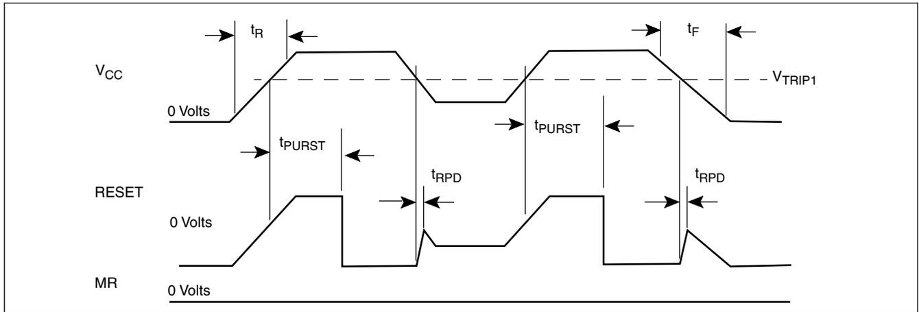
**Figure 31. Manual Reset Timing Diagram**
