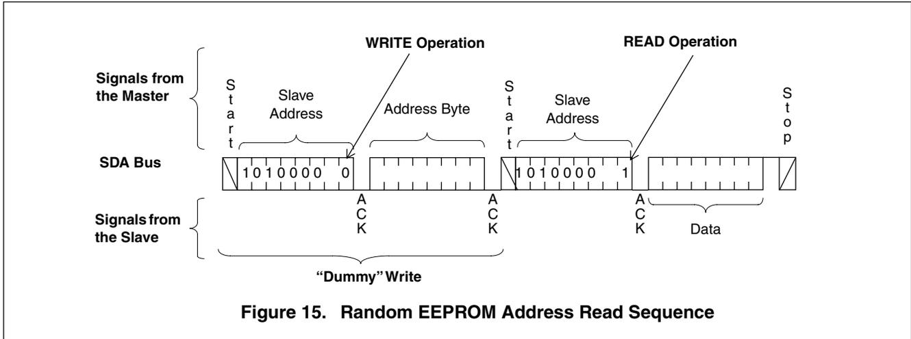
the Device Type Identifier 1010111 or 1010010). Immediately after an operation to a DCP or CR Register is performed, only a “Random EEPROM Read” is available. Immediately following a “Random EEPROM Read”, a “Current EEPROM Address Read” or “Sequential EEPROM Read” is once again available (assuming that no access to a DCP or CR Register occur in the interim).
