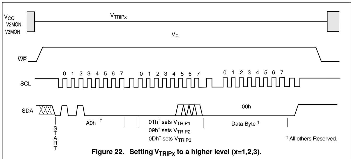
**Figure 22. Setting  $V_{TRIPx}$  to a higher level (x=1,2,3).**
