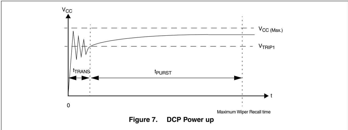
A nonvolatile write to a DCP will change the “wiper position” by simultaneously writing new data to the associated WCR and NVM. Therefore, the new “wiper position” setting is recalled into the WCR after  $V_{CC}$  of the X4023x is powered down and then powered back up.
