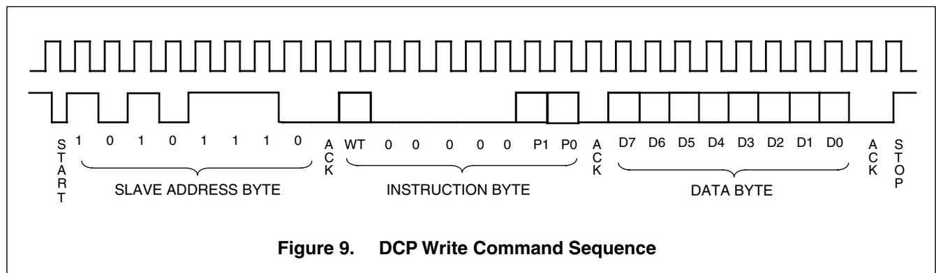
Figure 9. DCP Write Command Sequence
