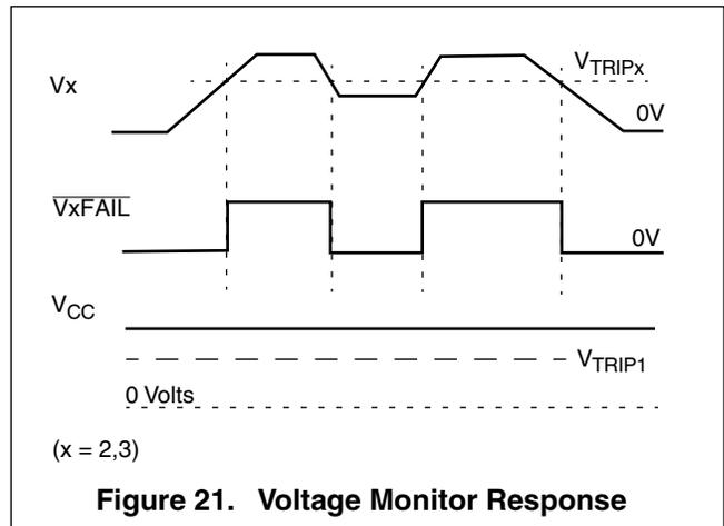
**Figure 21. Voltage Monitor Response**
