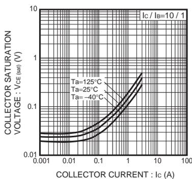
Fig.4 Collector-Emitter Saturation Voltage vs. Collector Current (I)
