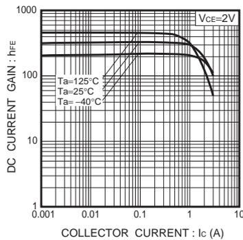
Fig.2 DC Current Gain vs. Collector Current (I)
