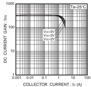
Fig.3 DC Current Gain vs. Collector Current (II)
