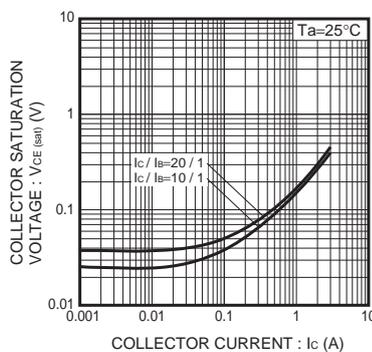
Fig.5 Collector-Emitter Saturation Voltage vs. Collector Current (II)
