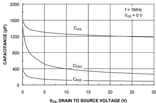
Figure 8. Capacitance Characteristics.
