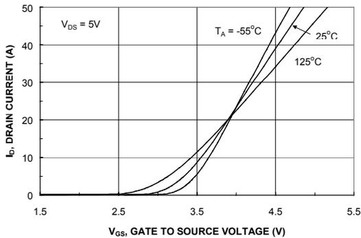
Figure 5. Transfer Characteristics.
