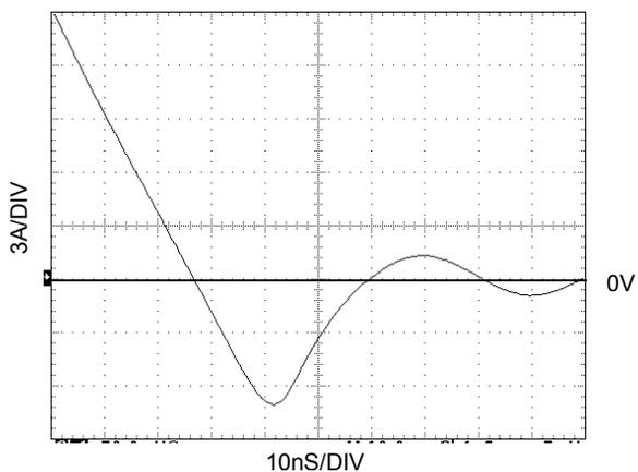
**Figure 13. Non-SyncFET (FDS6690A) body diode reverse recovery characteristic.**
