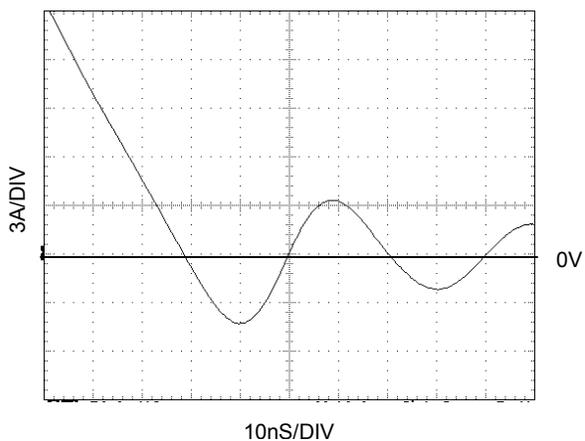
**Figure 12. FDS6690S SyncFET body diode reverse recovery characteristic.**
