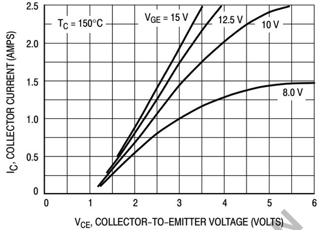
Figure 2. Saturation Characteristics
