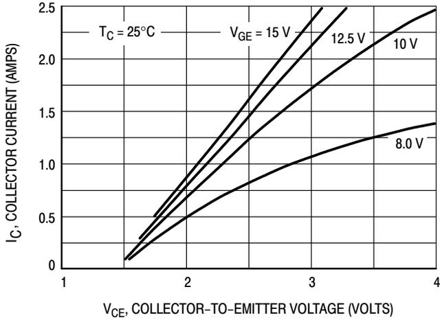
Figure 1. Saturation Characteristics
