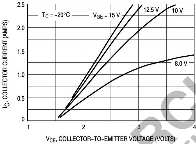
Figure 3. Saturation Characteristics
