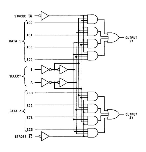
FIGURE 3. Logic diagram.
