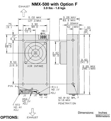
Option "F", Fan/Cover Assembly: Cover with integral ball-bearing fan provides proper cooling to achieve full ratings at 50°C ambient temperature. 2.05" dimension increases to 3.28".
