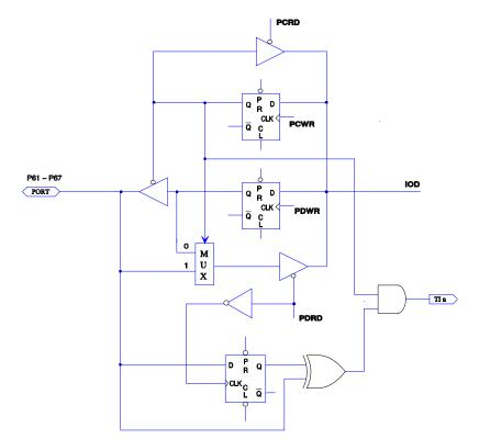
\*Pull-high (down), Open-drain are not shown in the figure.
