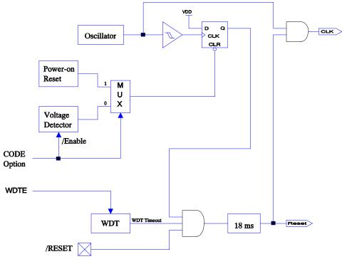
Fig. 9 Block diagram of Reset of controller
