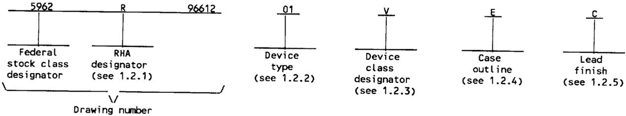
1.2.1 RHA designator. Device class M RHA marked devices shall meet the MIL-I-38535 appendix A specified RHA levels and shall be marked with the appropriate RHA designator. Device classes Q and V RHA marked devices shall meet the MIL-I-38535 specified RHA levels and shall be marked with the appropriate RHA designator. A dash (-) indicates a non-RHA device.
