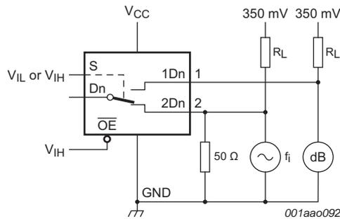
**Fig 15. Test circuit for measuring crosstalk**
