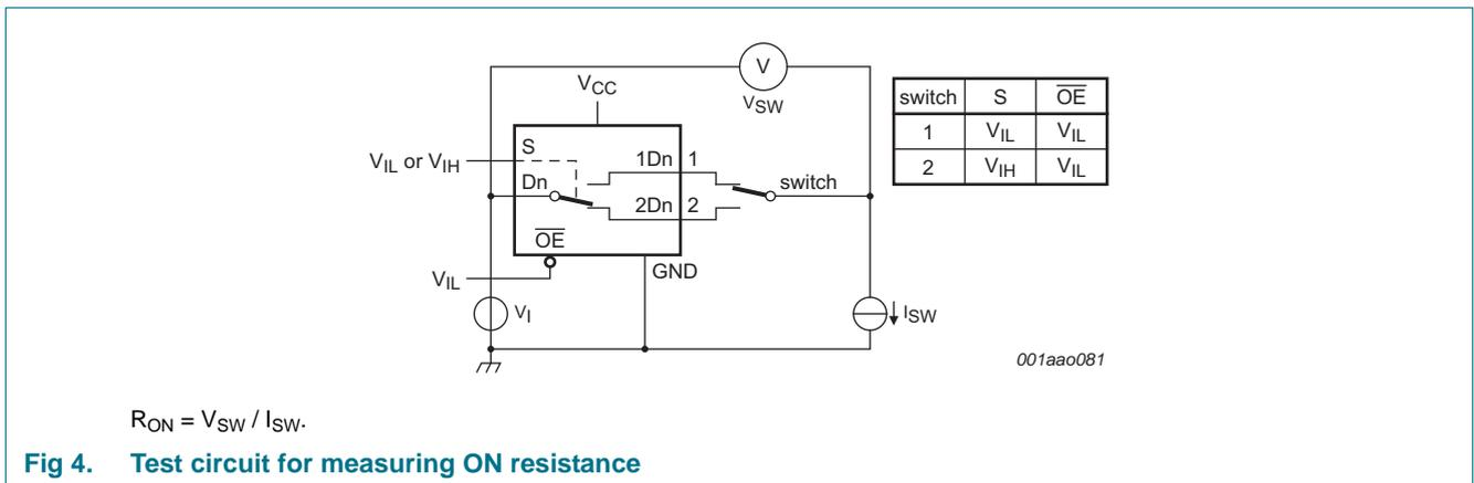
**Fig 4. Test circuit for measuring ON resistance**
