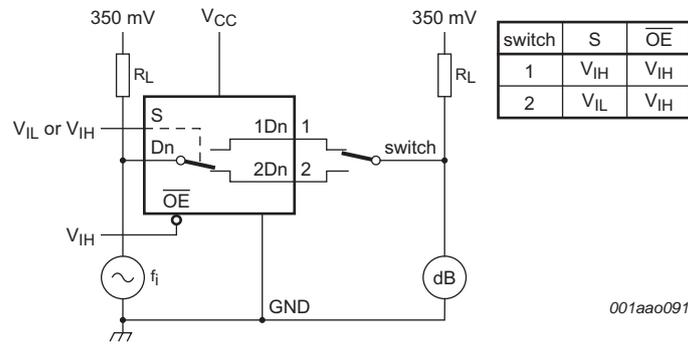
Adjust  $f_i$  voltage to obtain 0 dBm level at input.
