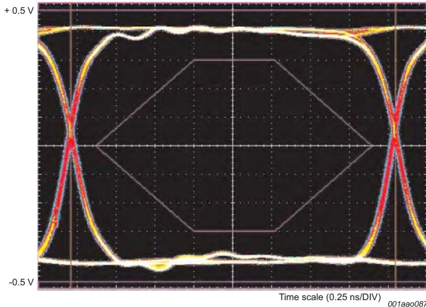
**Fig 10. Eye-pattern 480 Mbps USB signal with no switch.**
