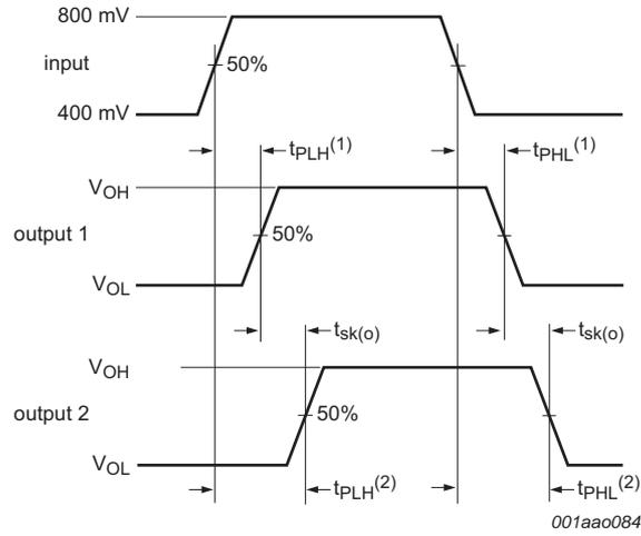
Logic levels:  $V_{OL}$  and  $V_{OH}$  are typical output voltage levels that occur with the output load.
