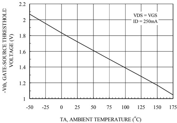
Figure 9.  $V_{th}$  Gate to Source Voltage Vs Temperature
