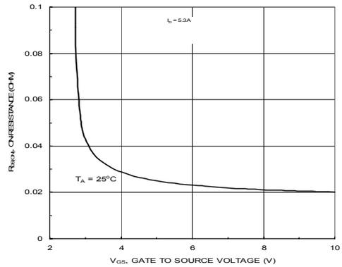
Figure 8. On-Resistance with Gate to Source Voltage
