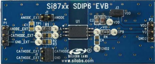
Figure 3. Si87xx SDIP6 Evaluation Board Overview
