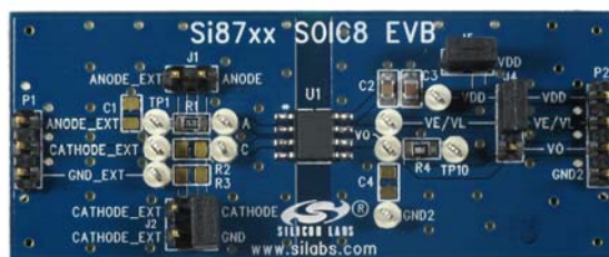
Figure 2. Si87xx SOIC8 Evaluation Board Overview
