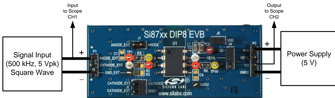
Figure 5. Summary Diagram and Test Setup
