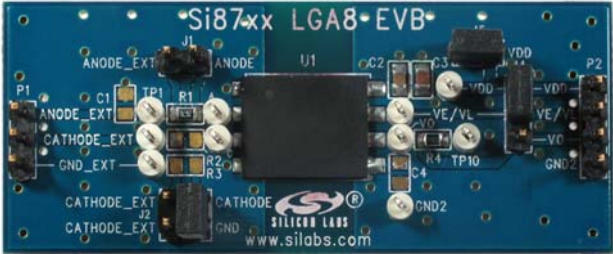
Figure 4. Si87xx LGA8 Evaluation Board Overview
