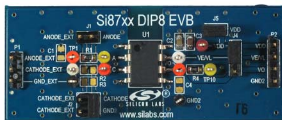
Figure 1. Si87xx DIP8 Evaluation Board Overview
