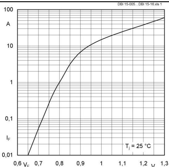
Fig. 1 : Forward characteristic (typical values)
