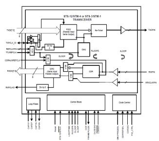
Ability to disable and bypass onchip CDR for external based received reference clock recovery thru
