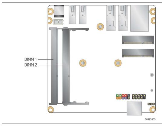
Figure 4. Memory Channel and SO-DIMM Configuration
