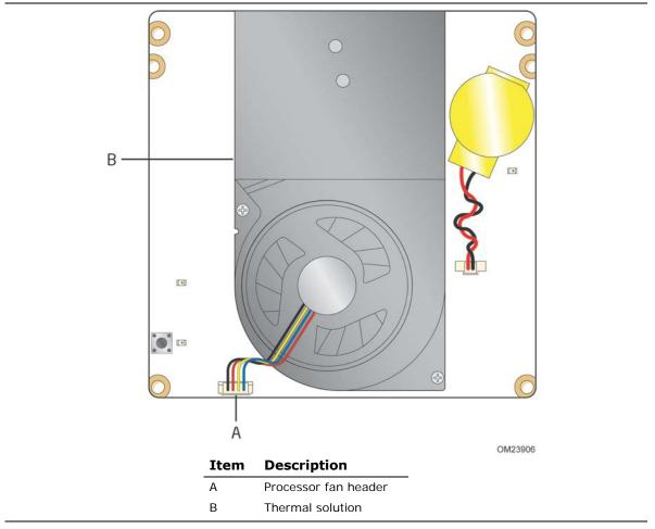
Figure 6. Thermal Solution and Fan Header
