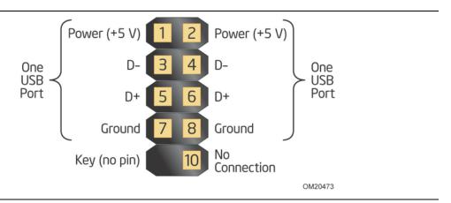
Figure 12. Connection Diagram for Front Panel USB 2.0 Dual-Port Header
