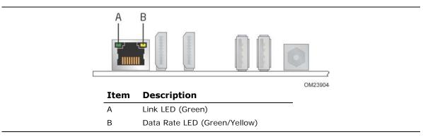
Figure 5. LAN Connector LED Locations
