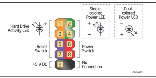
Figure 11. Connection Diagram for Front Panel Header
