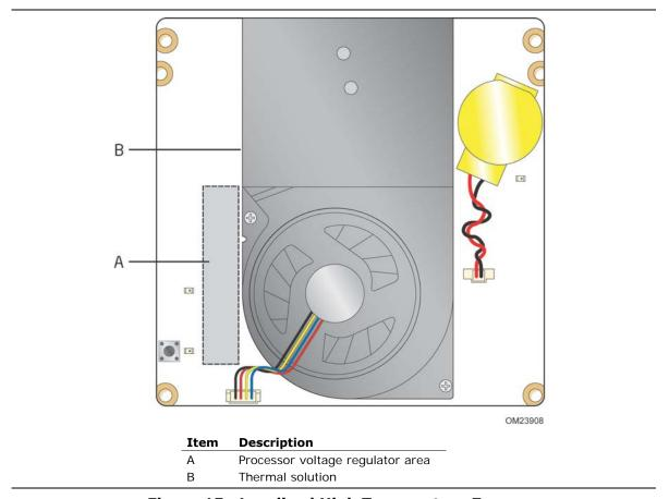
Figure 15. Localized High Temperature Zones
