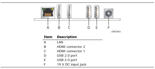
**Figure 9. Back Panel Connectors**
