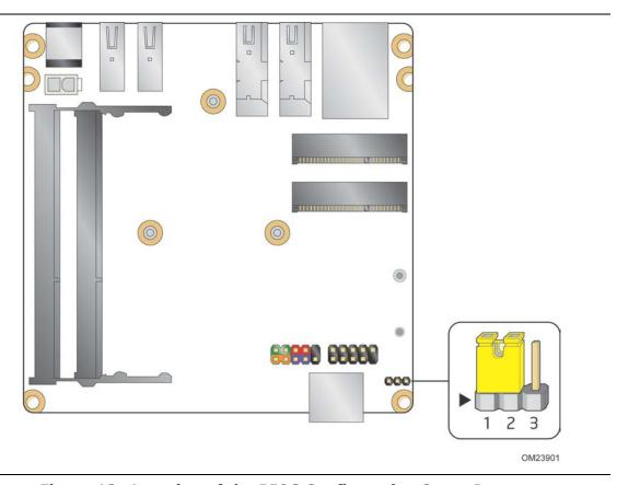
Figure 13. Location of the BIOS Configuration Setup Jumper
