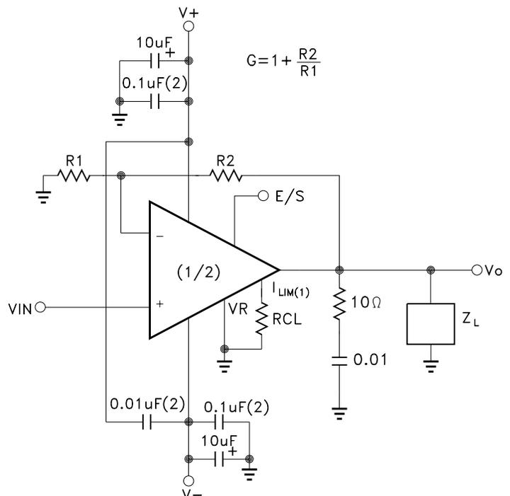
NOTE: (1) I<sub>LIM</sub> connected to VR achieves the maximum current limit, 10A(peak). (2) Connect capacitors directly to package power supply pins.
