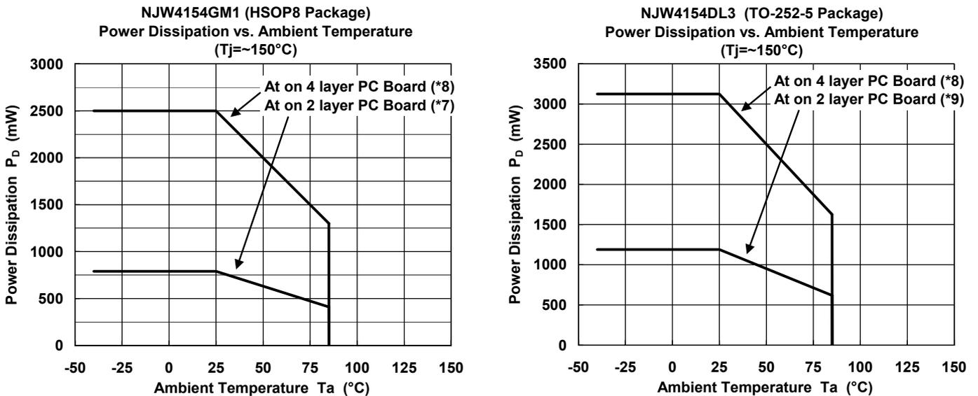
(\*7): Mounted on glass epoxy board. (76.2×114.3×1.6mm:based on EIA/JDEC standard, 2Layers)
