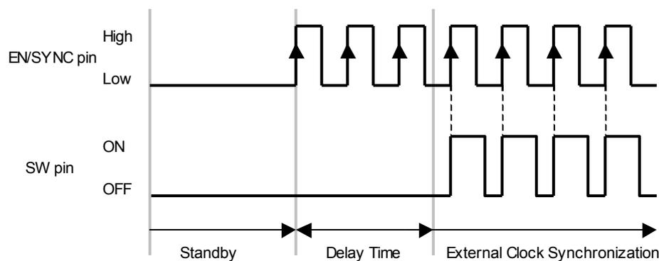
Fig. 3. Switching Operation by External Synchronized Clock
