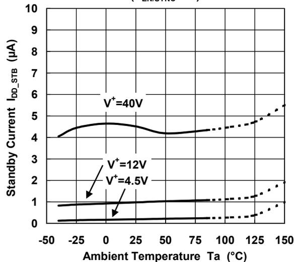
Switching Leak Current vs. Temperature
