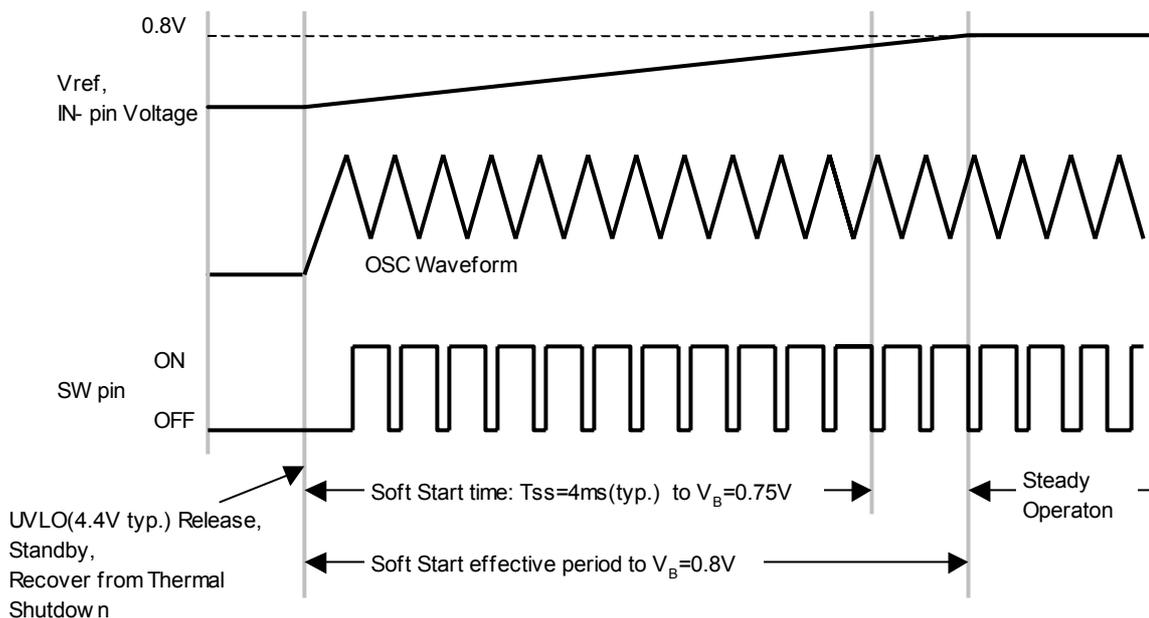
Fig. 1. Startup Timing Chart
