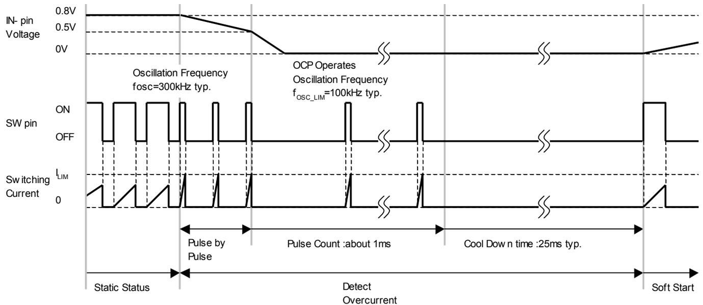
Fig. 2. Timing Chart at Over Current Detection
