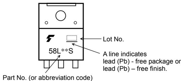
Note1: The “\*\*” in each product name is replaced with the output voltage of each product.
