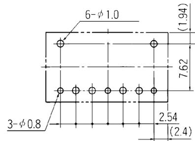
UM1L-D type (Double winding latching type)
