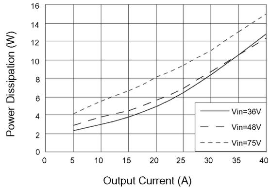
Fig.13 Typical power dissipation curve of ALQ-40G48N
