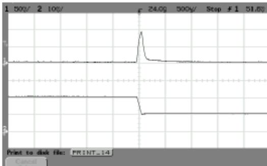
ALQ-40G48N Typical Transient Response to Step Decrease in Load from 50% to 25% of Full Load, Room Temperature, 48Vdc Input ( $\Delta I_o/\Delta t = 0.1A/1\mu s$ )
