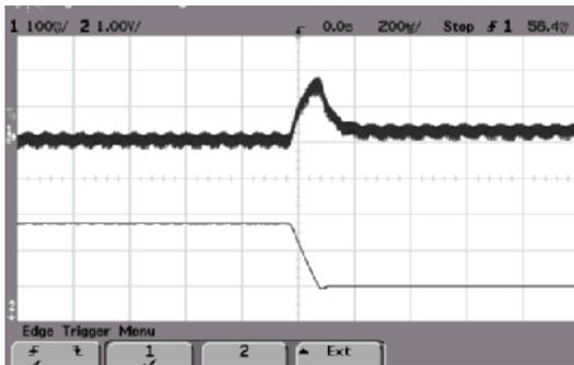
ALQ-35F48N Typical Transient Response to Step Decrease in Load from 50% to 25% of Full Load, Room Temperature, 48Vdc Input ( $\Delta I_o/\Delta t = 1A/1\mu s$ )
