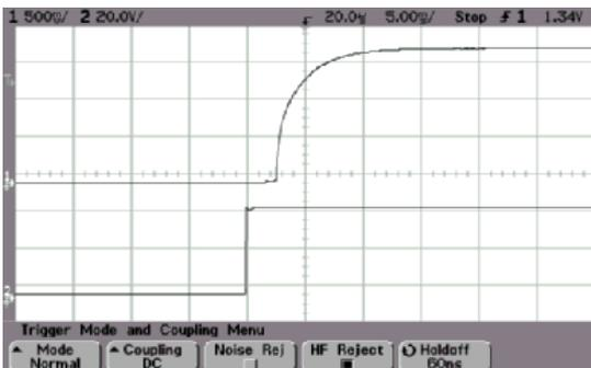
ALQ-40Y48N Typical Start-up from Power On
