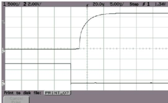
ALQ-40Y48N Typical Start-up from CNT On
