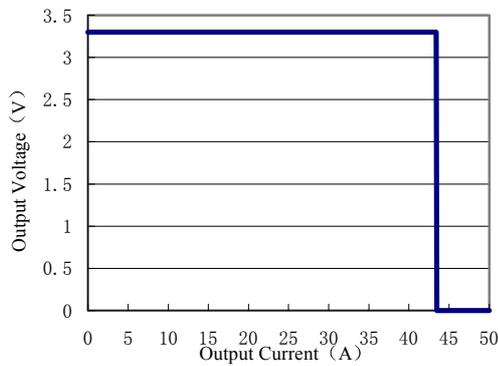
ALQ-35F48N Typical Output Over-current Curves
