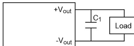
Fig.4 Output Ripple Filter
