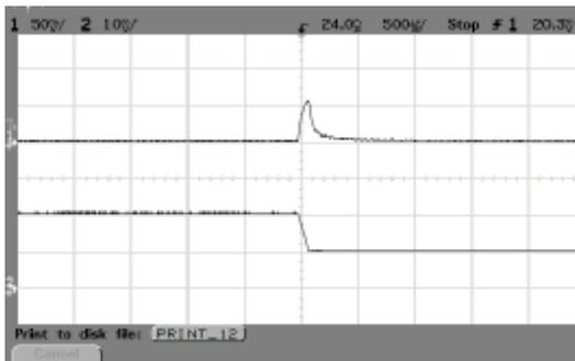
ALQ-40Y48N Typical Transient Response to Step Decrease in Load from 50% to 25% of Full Load, Room Temperature, 48Vdc Input ( $\Delta I_o/\Delta t = 0.1A/1\mu s$ )
