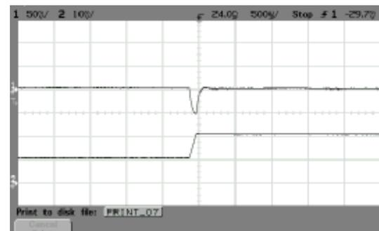
ALQ-40K48N Typical Transient Response to Step Increase in Load from 50% to 75% of Full Load, Room Temperature, 48Vdc Input ( $\Delta I_o/\Delta t = 0.1A/1\mu s$ )
