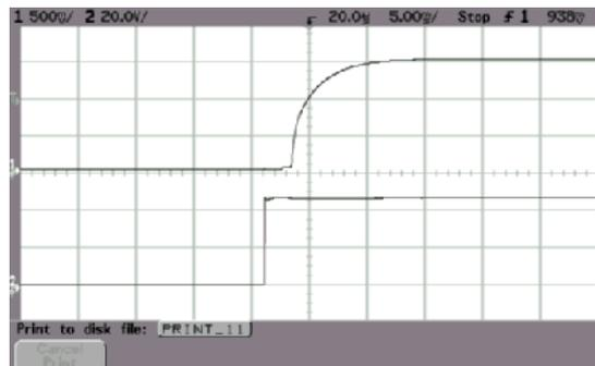
ALQ-40M48N Typical Start-up from Power On
