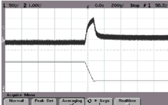
ALQ-40M48N Typical Transient Response to Step Decrease in Load from 50% to 25% of Full Load, Room Temperature, 48Vdc Input ( $\Delta I_o/\Delta t = 1A/1\mu s$ )
