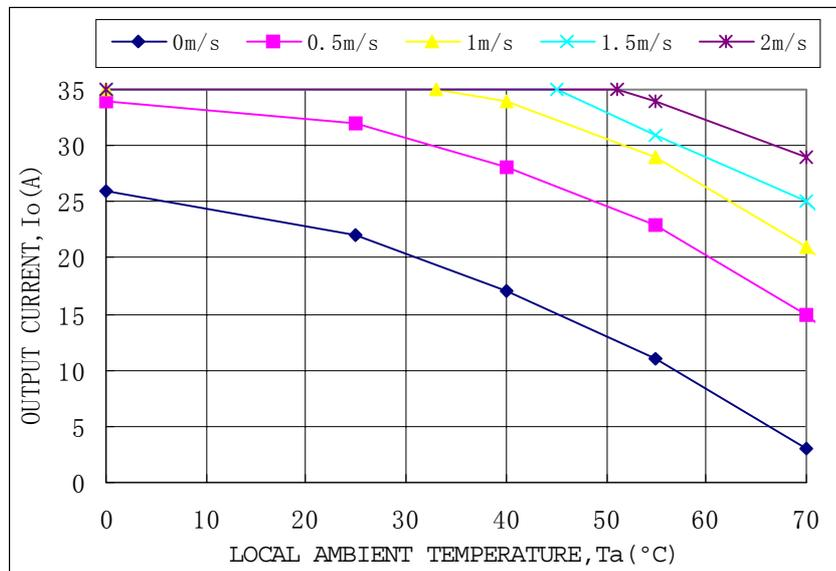
Fig.17 Output Power Derating for ALQ-35F48N (Vo = 3.3V)
