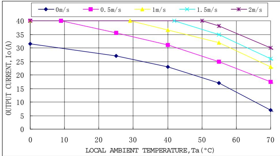
Fig.19 Output Power Derating for ALQ-40G48N (Vo = 2.5V)
