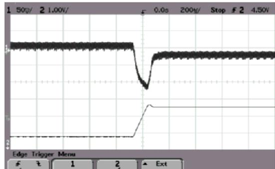
ALQ-40K48N Typical Transient Response to Step Increase in Load from 50% to 75% of Full Load, Room Temperature, 48Vdc Input ( $\Delta I_o/\Delta t = 1A/1\mu s$ )
