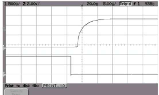
ALQ-40M48N Typical Start-up from CNT On
