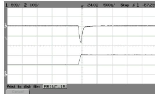
ALQ-40G48N Typical Transient Response to Step Increase in Load from 50% to 75% of Full Load, Room Temperature, 48Vdc Input ( $\Delta I_o/\Delta t = 0.1A/1\mu s$ )
