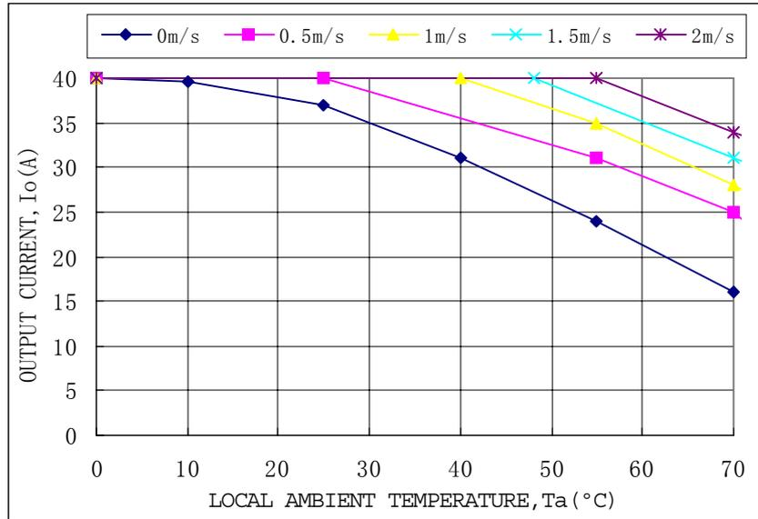
Fig.23 Output Power Derating for ALQ-40M48N ( $V_o = 1.5V$ )
