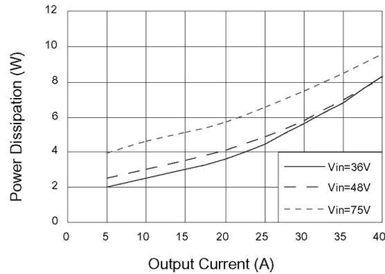
Fig.16 Typical power dissipation curve of ALQ-40K48N
