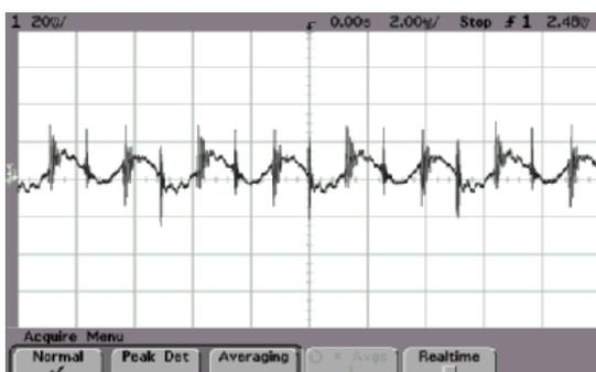
ALQ-40K48N Typical Output Ripple Voltage
