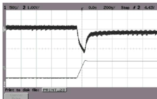
ALQ-40Y48N Typical Transient Response to Step Increase in Load from 50% to 75% of Full Load, Room Temperature, 48Vdc Input ( $\Delta I_o/\Delta t = 1A/1\mu s$ )
