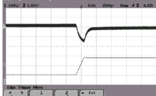
ALQ-40G48N Typical Transient Response to Step Increase in Load from 50% to 75% of Full Load, Room Temperature, 48Vdc Input ( $\Delta I_o/\Delta t = 1A/1\mu s$ )
