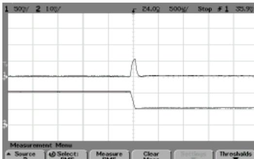
ALQ-40K48N Typical Transient Response to Step Decrease in Load from 50% to 25% of Full Load, Room Temperature, 48Vdc Input ( $\Delta I_o/\Delta t = 0.1A/1\mu s$ )
