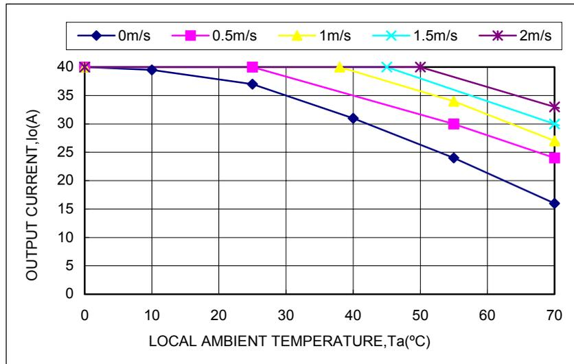
Figures24 Output Power Derating for ALQ-40M48N ( $V_o = 1.5V$ )
