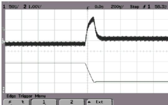
ALQ-40K48N Typical Transient Response to Step Decrease in Load from 50% to 25% of Full Load, Room Temperature, 48Vdc Input ( $\Delta I_o/\Delta t = 1A/1\mu s$ )
