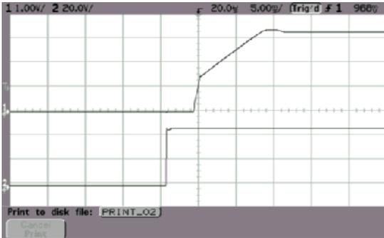
ALQ-35F48N Typical Start-up from Power On
