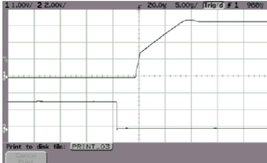
ALQ-35F48N Typical Start-up from CNT On
