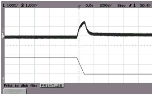
ALQ-40G48N Typical Transient Response to Step Decrease in Load from 50% to 25% of Full Load, Room Temperature, 48Vdc Input ( $\Delta I_o/\Delta t = 1A/1\mu s$ )
