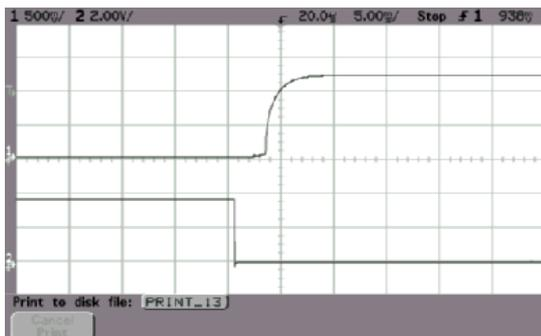
ALQ-40K48N Typical Start-up from CNT On
