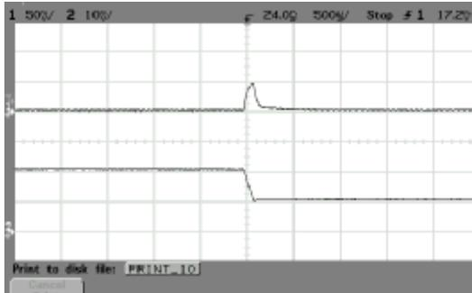
ALQ-40M48N Typical Transient Response to Step Decrease in Load from 50% to 25% of Full Load, Room Temperature, 48Vdc Input ( $\Delta I_o/\Delta t = 0.1A/1\mu s$ )
