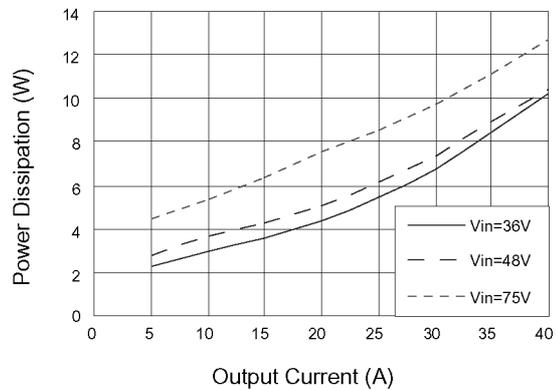
Fig.14 Typical power dissipation curve of ALQ-40Y48N
