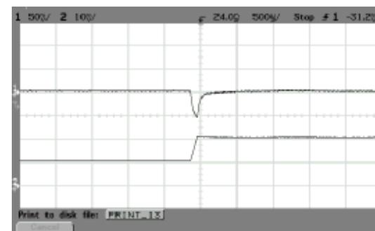
ALQ-40Y48N Typical Transient Response to Step Increase in Load from 50% to 75% of Full Load, Room Temperature, 48Vdc Input ( $\Delta I_o/\Delta t = 0.1A/1\mu s$ )
