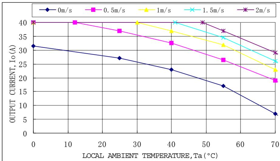
Fig.20 Output Power Derating for ALQ-40G48N (Vo = 2.5V)
