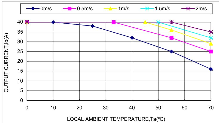
Figures 25 Output Power Derating for ALQ-40K48N (Vo = 1.2V)
