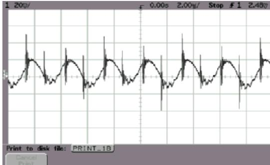
ALQ-35F48N Typical Output Ripple Voltage
