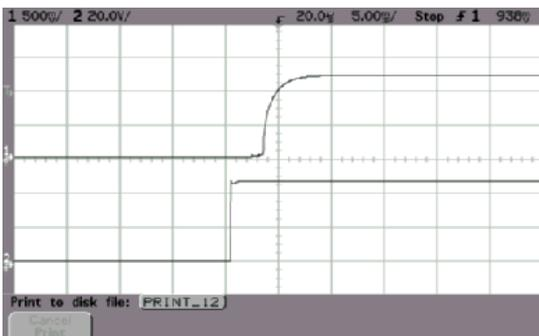
ALQ-40K48N Typical Start-up from Power On
