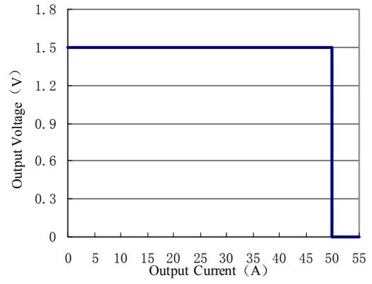
ALQ-40Y48N Typical Output Over-current Curves
