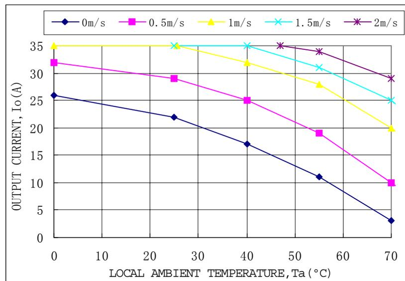
Fig.18 Output Power Derating for ALQ-35F48N (Vo = 3.3V)
