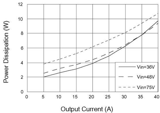
Fig.15 Typical power dissipation curve of ALQ-40M48N
