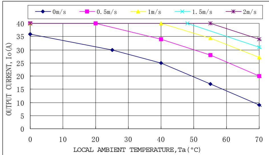
Fig.21 Output Power Derating for ALQ-40Y48N (Vo = 1.8V)
