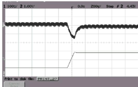
ALQ-35F48N Typical Transient Response to Step Increase in Load from 50% to 75% of Full Load, Room Temperature, 48Vdc Input ( $\Delta I_o/\Delta t = 1A/1\mu s$ )
