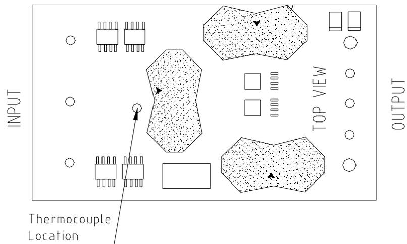
Fig.11 Temperature Measurement Location
