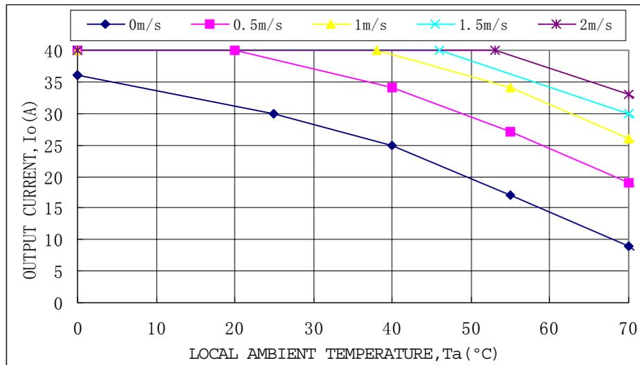
Fig.22 Output Power Derating for ALQ-40Y48N (Vo = 1.8V)
