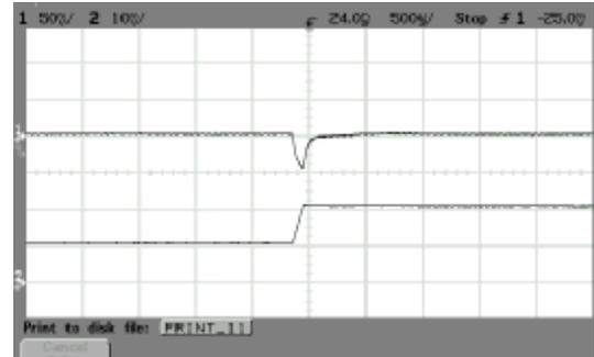
ALQ-40M48N Typical Transient Response to Step Increase in Load from 50% to 75% of Full Load, Room Temperature, 48Vdc Input ( $\Delta I_o/\Delta t = 0.1A/1\mu s$ )
