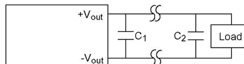
Fig.5 Output Ripple Filter for a Distant Load
