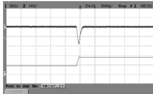
ALQ-35F48N Typical Transient Response to Step Increase in Load from 50% to 75% of Full Load, Room Temperature, 48Vdc Input ( $\Delta I_o/\Delta t = 0.1A/1\mu s$ )
