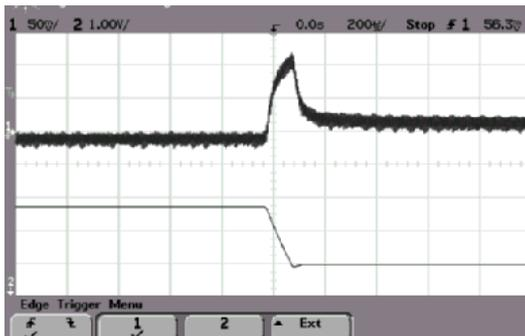
ALQ-40Y48N Typical Transient Response to Step Decrease in Load from 50% to 25% of Full Load, Room Temperature, 48Vdc Input ( $\Delta I_o/\Delta t = 1A/1\mu s$ )
