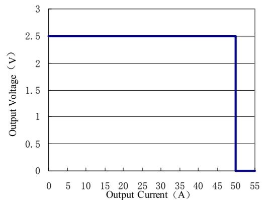
ALQ-40G48N Typical Output Over-current Curves
