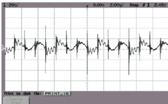
ALQ-40Y48N Typical Output Ripple Voltage
