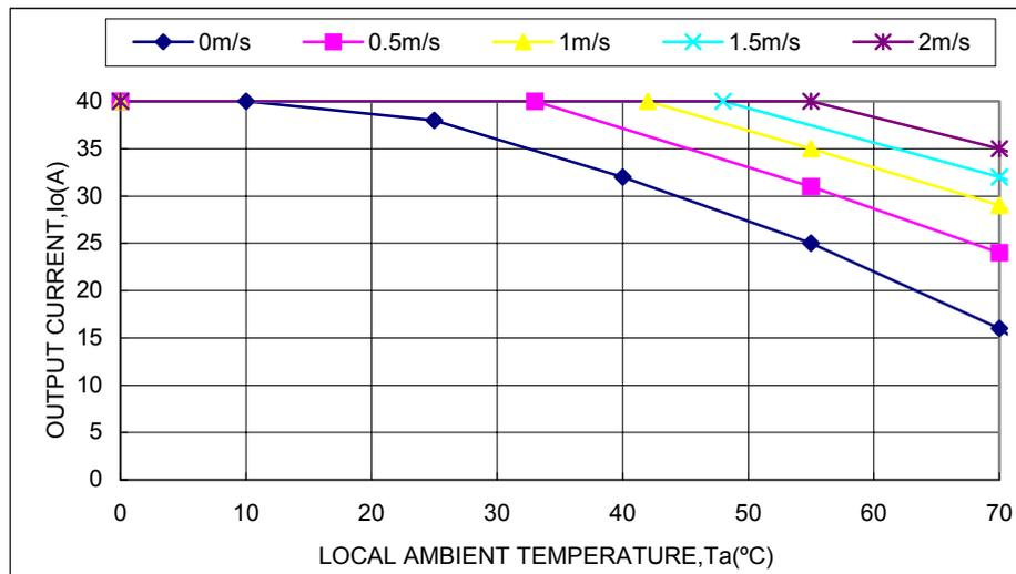
Figures 26 Output Power Derating for ALQ-40K48N (Vo = 1.2V)
