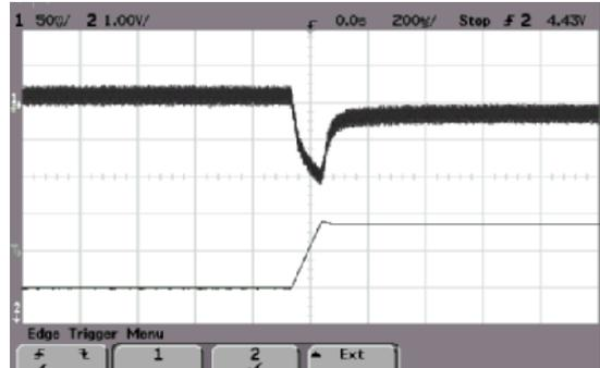
ALQ-40M48N Typical Transient Response to Step Increase in Load from 50% to 75% of Full Load, Room Temperature, 48Vdc Input ( $\Delta I_o/\Delta t = 1A/1\mu s$ )
