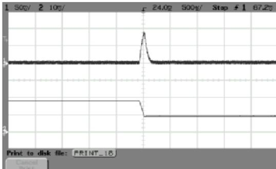
ALQ-35F48N Typical Transient Response to Step Decrease in Load from 50% to 25% of Full Load, Room Temperature, 48Vdc Input ( $\Delta I_o/\Delta t = 0.1A/1\mu s$ )
