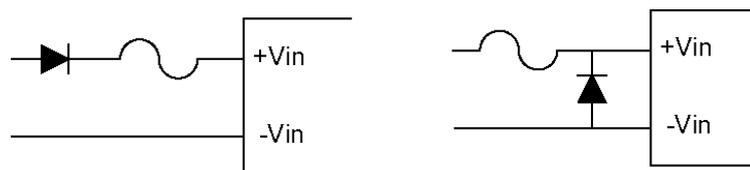
Fig.9 Reverse Polarity Protection Circuit
