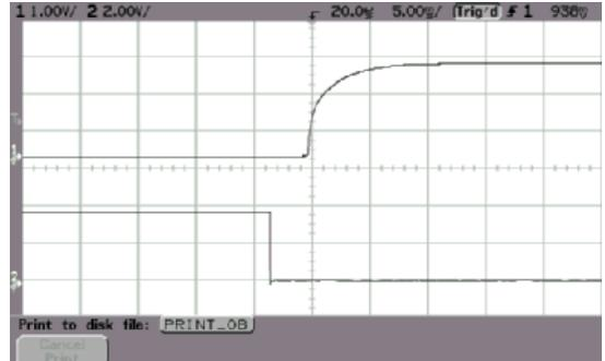
ALQ-40G48N Typical Start-up from CNT On
