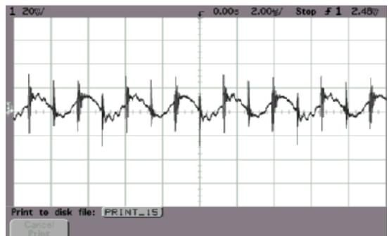
ALQ-40M48N Typical Output Ripple, Voltage
