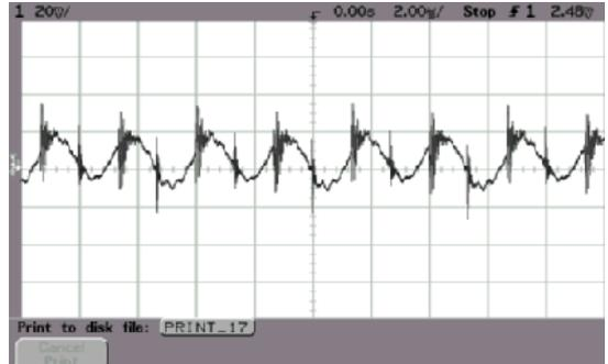
ALQ-40G48N Typical Output Ripple Voltage
