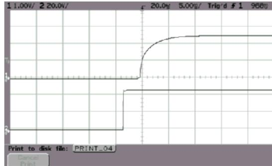
ALQ-40G48N Typical Start-up from Power On
