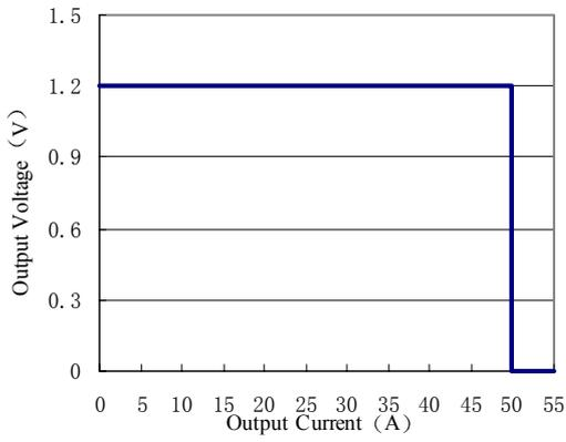
ALQ-40K48N Typical Output Over-current Curves
