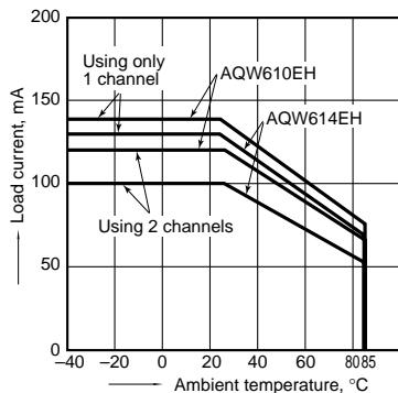
1-(2). Load current vs. ambient temperature characteristics
