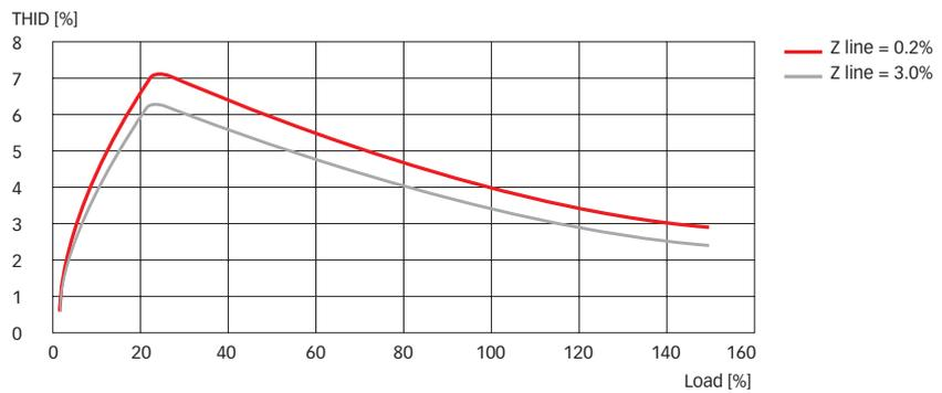
**High performance – not only at full load.** Often manufacturers promote filter performance only at full load because light load conditions can be a challenge in terms of both harmonics mitigation and capacitive current. Schaffner ECOSine™ filters not only guarantee the THID rating of 8% maximum over the entire load range, but also limit the amount of capacitive current in all conditions.
