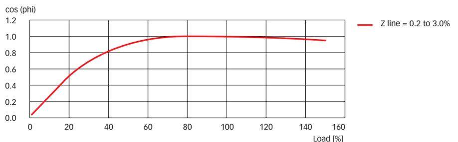
An external capacitor disconnect switch can easily be installed, if capacitive current under light load conditions has to be suppressed. You can obtain more information on this subject from the Schaffner ECOSine™ application note.
