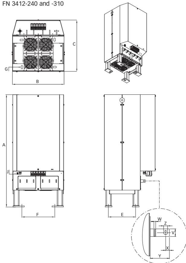
**Installation.** All filters from FN 341x-8 to -130 are wall mountable and have to be operated vertically. The filters FN 341x-150 and higher are designed for floor mounting. In order to allow for sufficient air flow all filters must be clear on top and bottom min. 150mm.
