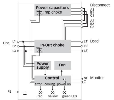
\* ECOSine filters reduce RMS input and peak current by reducing harmonic currents and improving true power factor.
