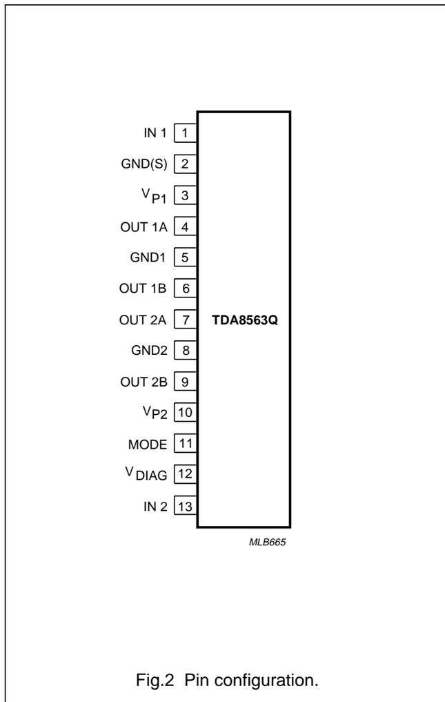
Fig.2 Pin configuration.
