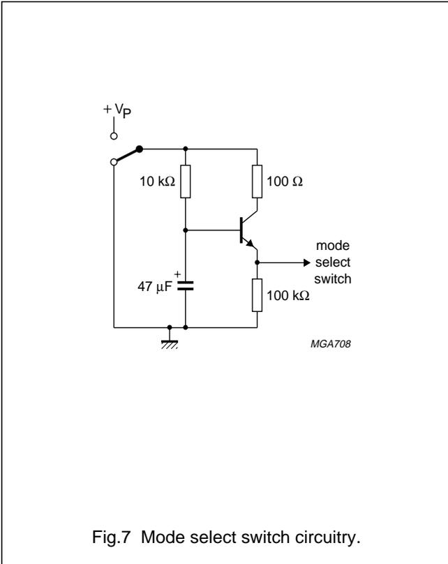
Fig.7 Mode select switch circuitry.
