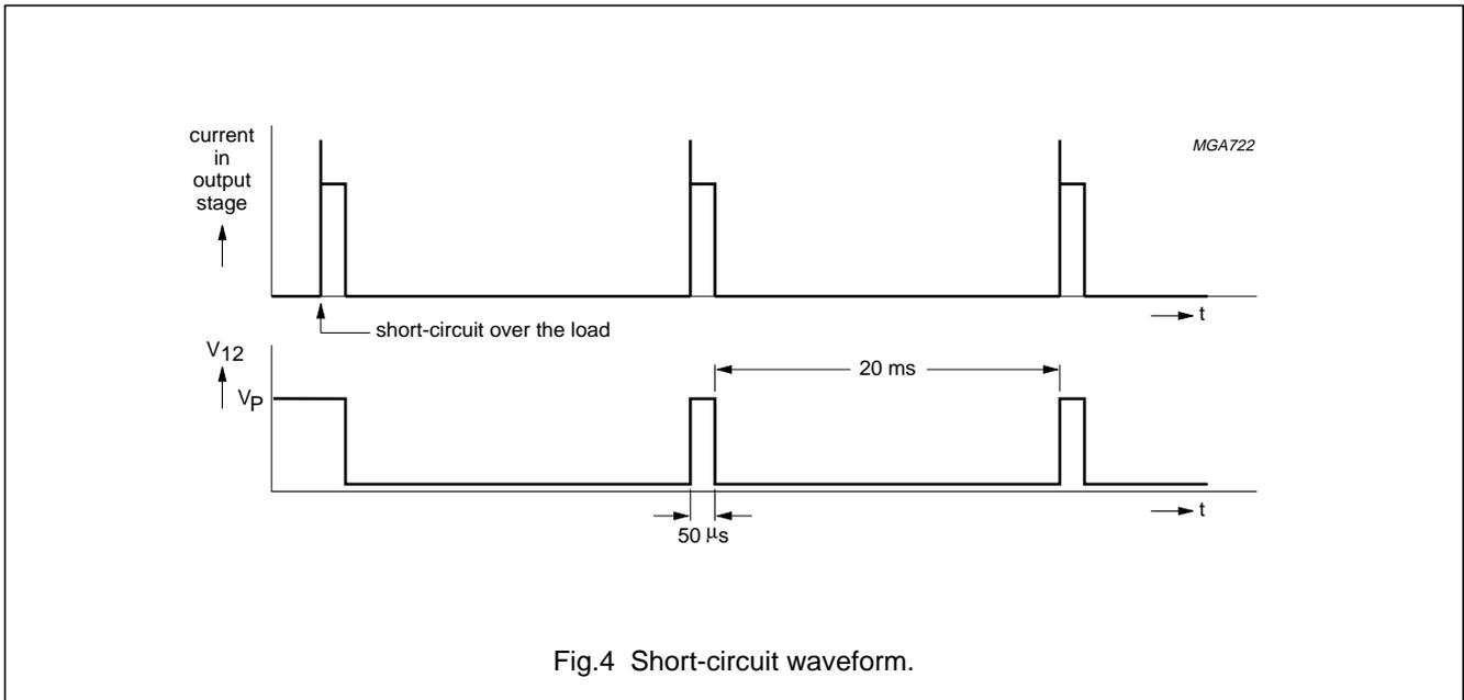
Fig.4 Short-circuit waveform.
