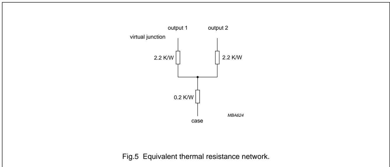
Fig.5 Equivalent thermal resistance network.
