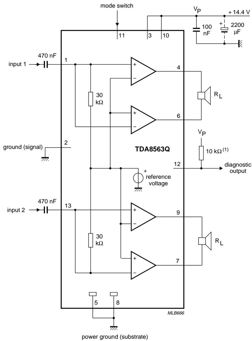
(1) To avoid high energy switching pulses which can feedback to the inputs it is advisable to ensure that the value of the resistor at pin 12 is  $\geq 10 \text{ k}\Omega$ .
