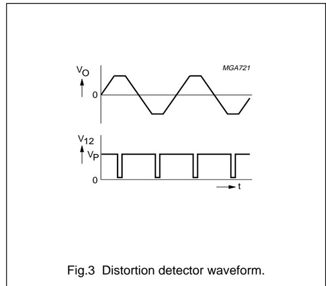
Fig.3 Distortion detector waveform.
