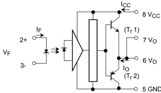
(Note 2) A 0.1  $\mu$ F bypass capacitor must be connected between pin 8 and 5.
