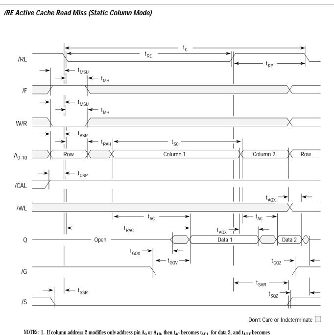
NOTES: 1. If column address 2 modifies only address pin  $A_9$  or  $A_{10}$ , then  $t_{AC}$  becomes  $t_{AC1}$  for data 2, and  $t_{AQX}$  becomes  $t_{AQX1}$  for data 1.
