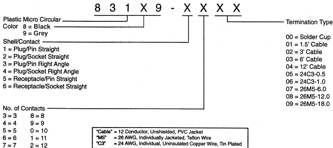
\* Recommended configuration is socket contacts in the receptacle connector, pin contacts in the plug connector.
