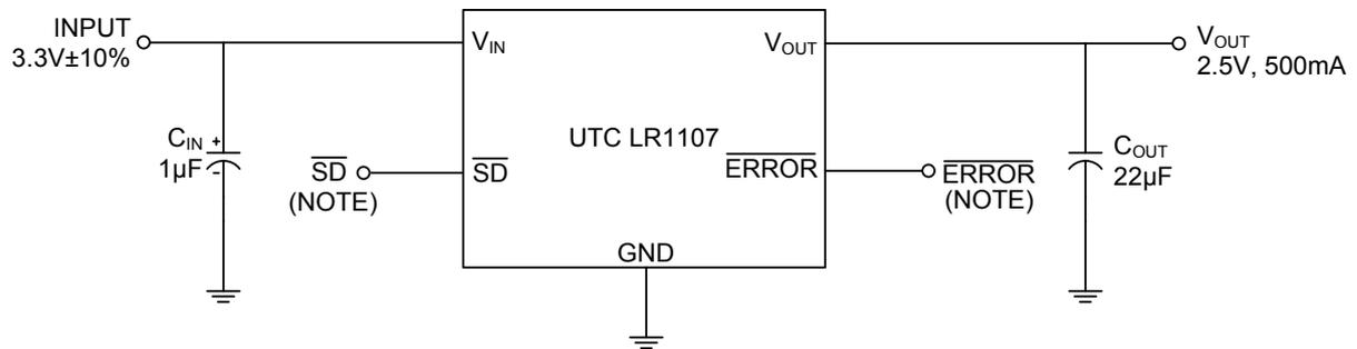
Note:  $\overline{SD}$  and  $\overline{ERROR}$  pins must be pulled high through a 10kΩ pull-up resistor. Connect the  $\overline{ERROR}$  pin to ground if this function is not used.
