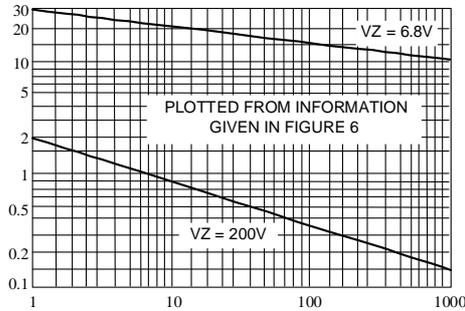
Fig. 6-PEAK SURGE CURRENT VERSUS PULSE WIDTH(SEE NOTE 3)
