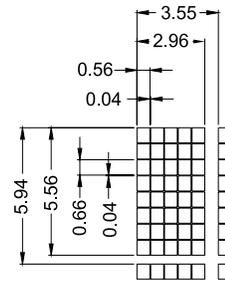
The tolerance unless classified  $\pm 0.3\text{mm}$
