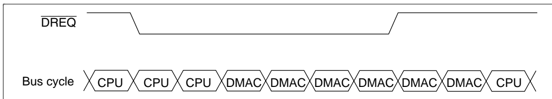
Figure 11.13 DMA Transfer Example in the Burst Mode
