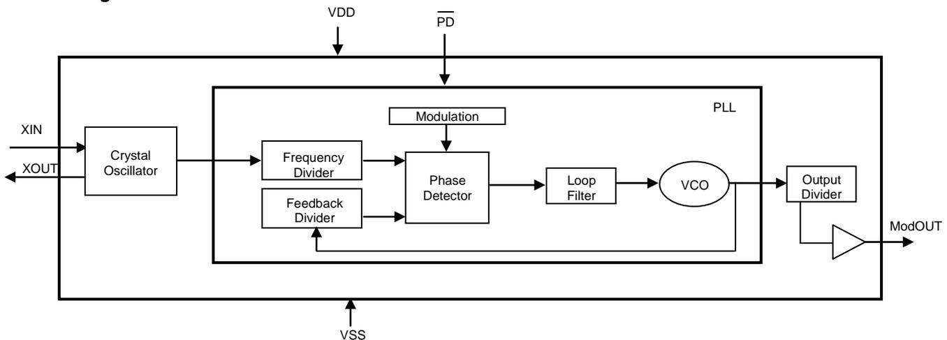
The ASM3P2760A uses the most efficient and optimized modulation profile approved by the FCC and is implemented by using a proprietary all digital method.
