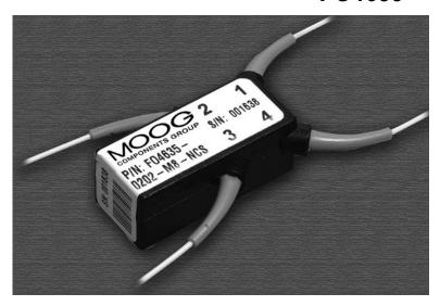
The silicon micromachine based electromechanical multimode switch uses a movable mirror process to allow light to pass through the switch on activation or to be blocked/diverted when the switch is deactivated. This makes the switch particularly well suited for fail-safe bypass applications.
