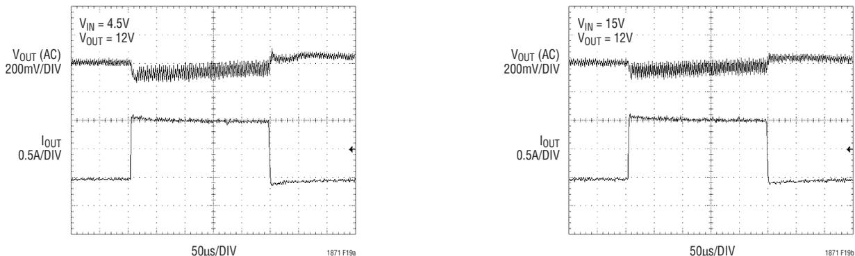
Figure 19. LTC1871-1 SEPIC Converter Load Step Response
