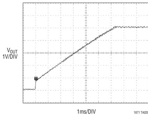
Load Step Response at  $V_{IN} = 4.5V$
