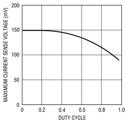
Figure 10. Maximum SENSE Threshold Voltage vs Duty Cycle
